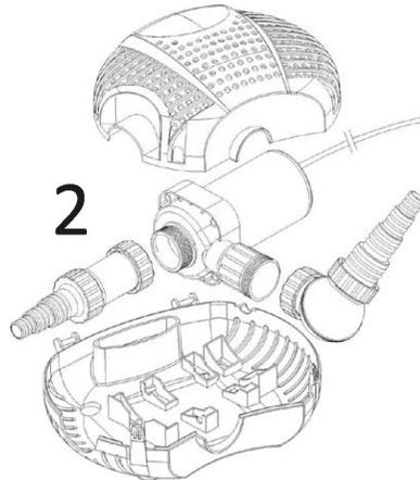
Open pump cover and remove pump
